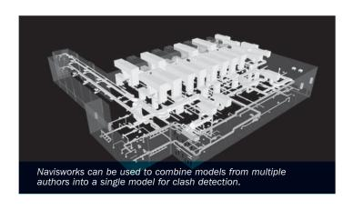
Why is clash detection so important? Because once it's time to build in the field, it's physically impossible to have two things in the same exact space. This means that an unresolved clash in the model would force a field crew to either make modifications, which takes time and could have unintended consequences later down the line, or stop work because the clash can't be easily resolved.
