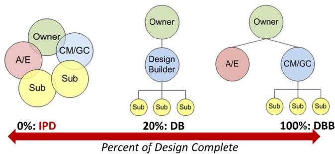
Fig. 1. Differences between DB, DBB, and IPD
